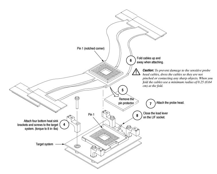
Figure 1-4: Attach the probe head to the target system
