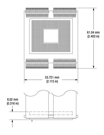
Figure 2-6: Dimensions of the probe head
