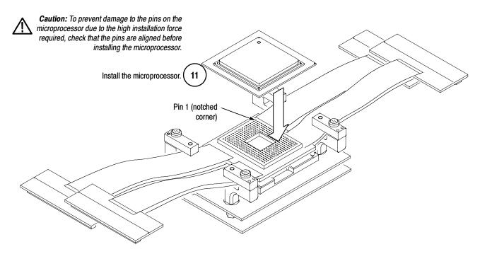
Figure 1-5: Attaching the heat sink brackets and microprocessor to the target system
