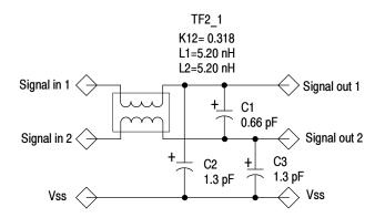
Figure 2-3: Socket electrical load model for typical signals
