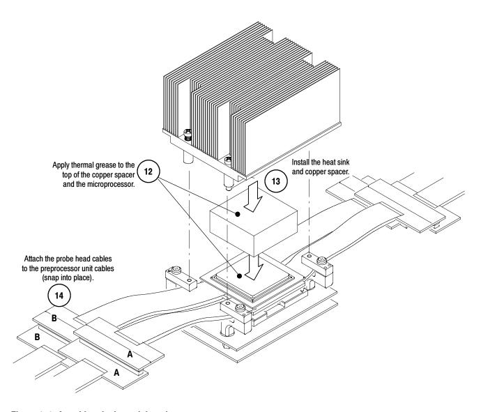
Figure 1-6: Attaching the heat sink to the target system
