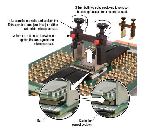
Figure 1-7: Remove the microprocessor with the extraction tool
