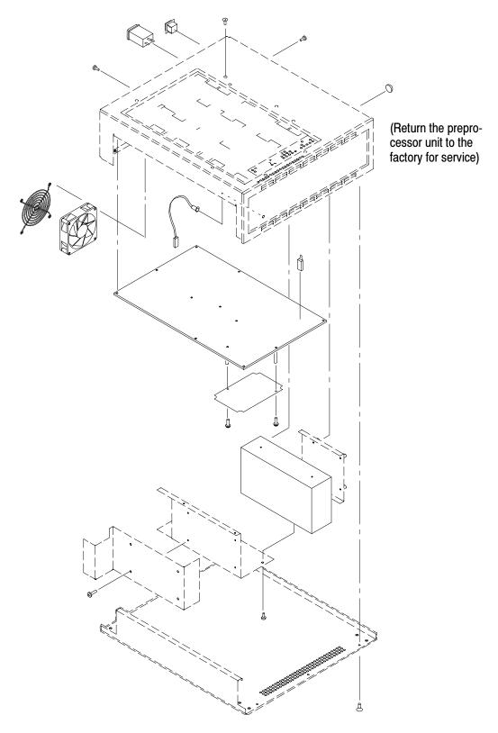
Figure 4-2: Preprocessor unit exploded view
