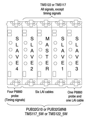
Figure 1-10: LAI cable, P6860 probe, and module configurations
