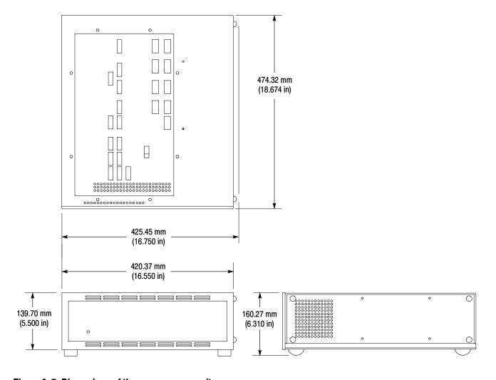
Figure 2-7: Dimensions of the preprocessor unit
