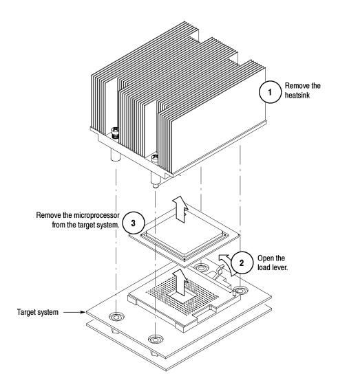
Figure 1-3: Removing microprocessor probe head from the target system
