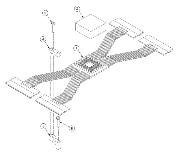
Figure 4-1: Probe adapter exploded view
